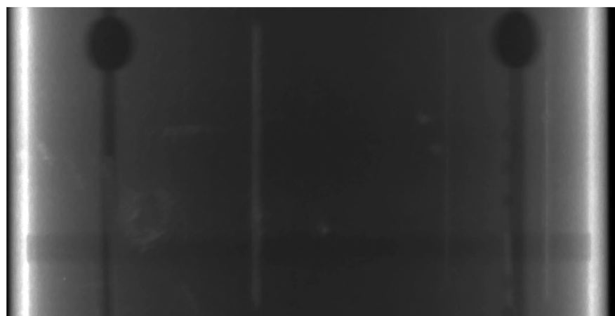
Figure 8 - Projection with intensities of unabsorbed radiation for an angle of -45 degrees DOI: https://doi.org/10.60797/itech.2026.12.3.8
